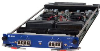
Modular blade technology allows for quick reconfiguration of chassis.
